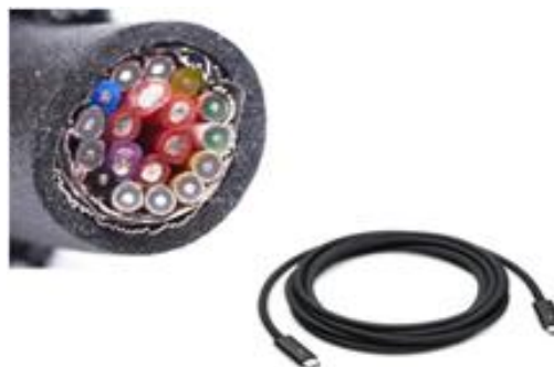
Figure 4: Thunderbolt 4 Transmission Cable (Outer Diameter 5.24mm)
